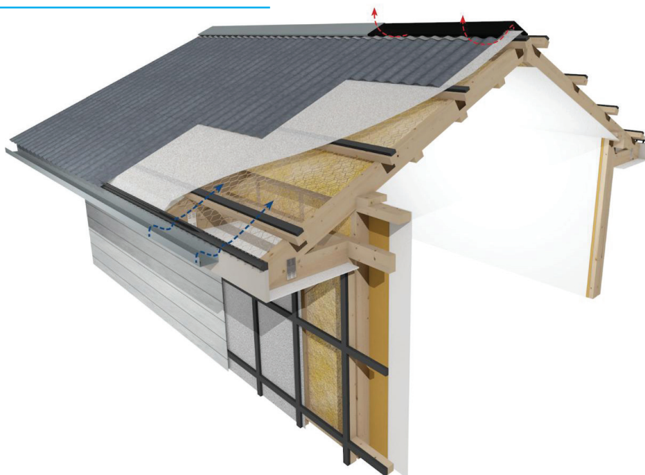
Fig A: 3D Render of VENT SYSTEMS VB20 Wall Cavity Battens in use with VENT SYSTEMS Passive Ventilation
