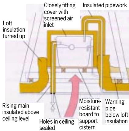
**Figure 2** Insulate pipes and cisterns in the roof space
