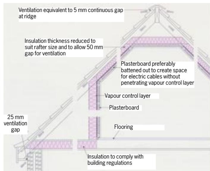
**Figure 8** How to ventilate the roof space round an attic room
