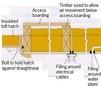
**Figure 1** Seal gaps round the loft hatch and service penetrations
