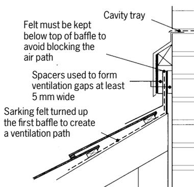
**Figure 9** Providing high level ventilation for a monopitch roof
