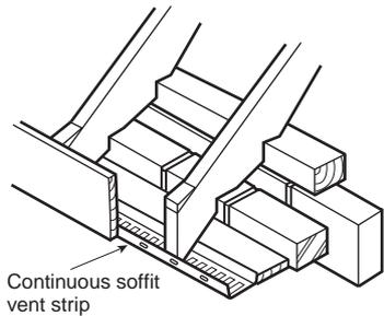
Continuous soffit vent strip
