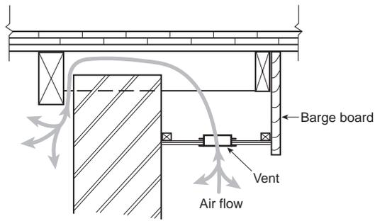
**Figure 5** Using boxed eaves as roof ventilation ducts
