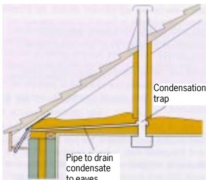
**Figure 3** Insulate ducts passing through the roof space
