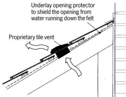
**Figure 6** Typical slope ventilator
