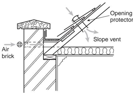
**Figure 10** Possible method for ventilating a parapet roof
