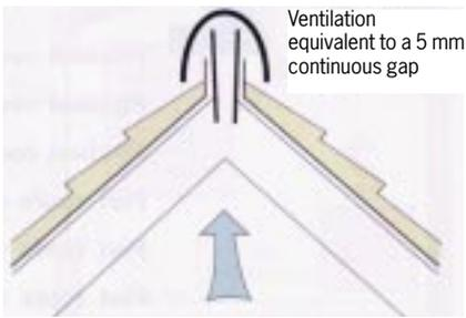
**Figure 7** Ridge ventilation in wide or steep pitch roofs
