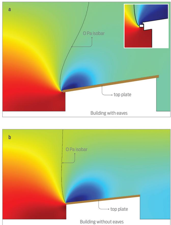
Figure 1: Air pressures on a monopitch skillion roof, (a) with and (b) without eaves. Dark red is high positive pressure, dark blue is high negative pressure.
