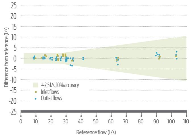
Figure 2: Measurement errors of a powered or active flow hood. The shaded area indicates the acceptable accuracy range.
