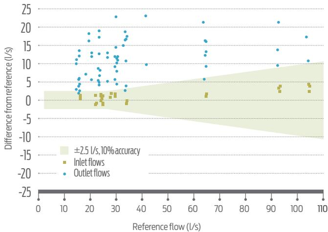
Figure 1: Measurement errors of a non-powered or passive flow hood. The shaded area indicates the acceptable accuracy range.
