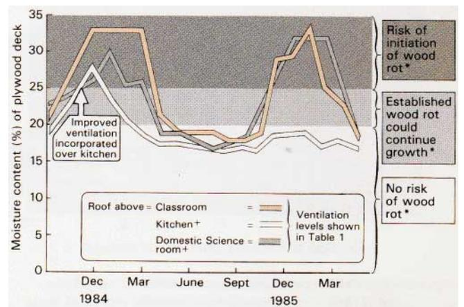
**Figure 4** School roofs: cyclical pattern of moisture content of plywood decks. For each roof, continuous data are shown for the monitored position which on average recorded the highest moisture content throughout the study.
