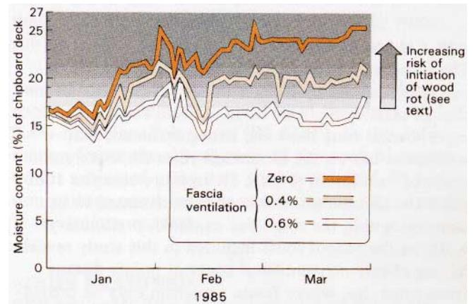
**Figure 3** Test roof: moisture contents of chipboard deck with different levels of ventilation. Continuous data are presented for a single location in an equivalent position in each roof cavity. Note: Fascia ventilation is provided only at one end of the roof cavity and one cowl vent (0.06% of plan area) is open in each case (configuration C in Figure 2)
