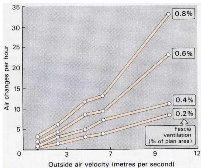
Figure 5 Test roof: air exchange rates for different ventilation levels and wind speeds (mean values for replicated tests)
