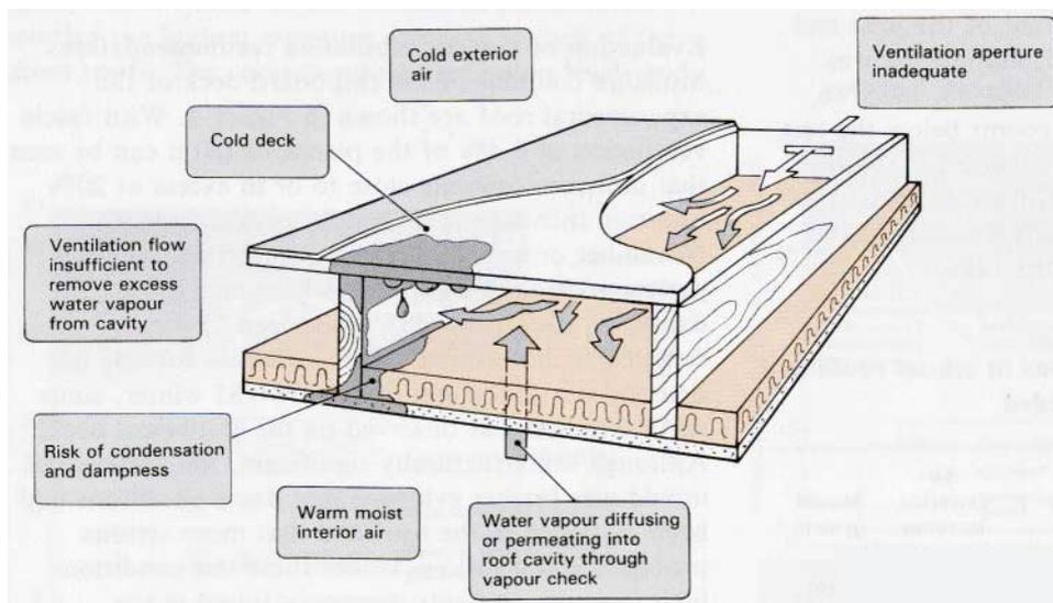
**Figure 1** Inadequate ventilation has serious consequences for cold deck flat roofs
