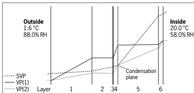
**Figure 1** Saturated vapour pressure and vapour pressure profiles through a timber framed wall
