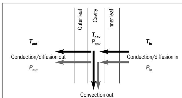
**Figure 2** Heat and moisture flows into and out of a cavity
