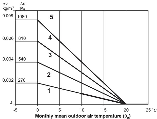
**Figure 4** Variation of internal humidity classes with external temperature for five different types of building occupancy
